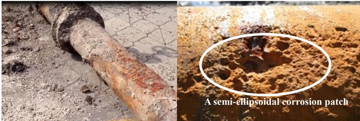
Figure 2. A corrosion patch formed on the external surface of a cast iron pipe
