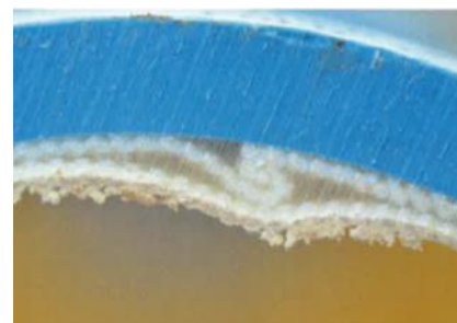
Type III - Only the outer fabric layer folds over to form a ridge
