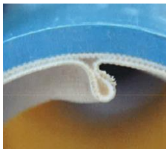
Type II - Only the inner layer moves upward and the space between the two fabric layers is filled with epoxy to form a ridge
