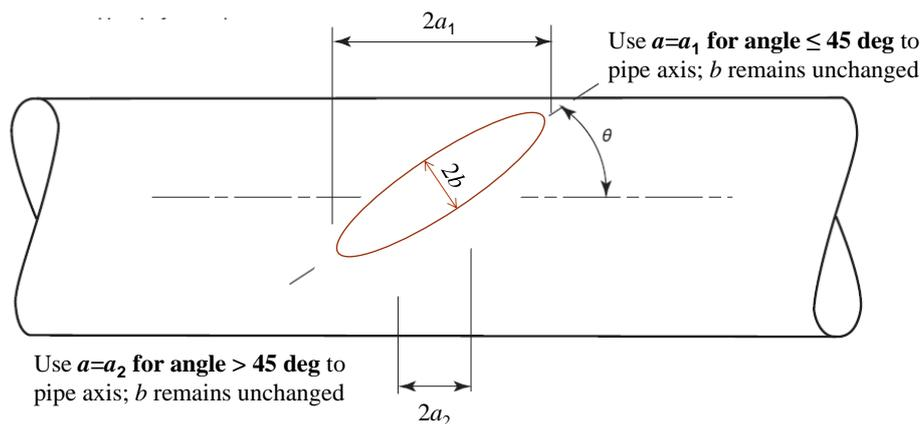
Figure 12. Change of length,  $2a$ , for an oriented corrosion defect
