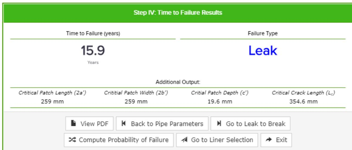
(b) Corrosion patch with dimensions ( $2a = 100$  mm,  $2b = 100$  mm,  $c = 18$  mm)
