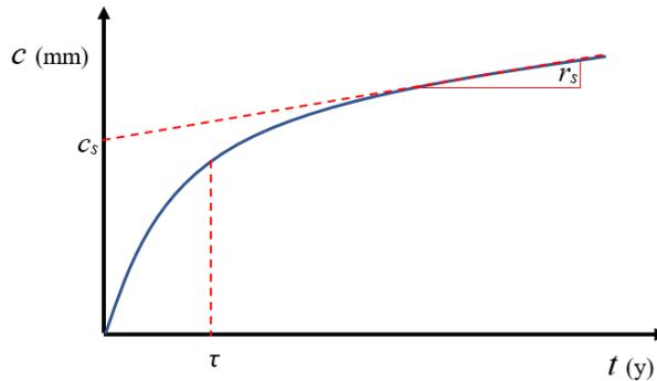
Figure 21. Exponential corrosion model
