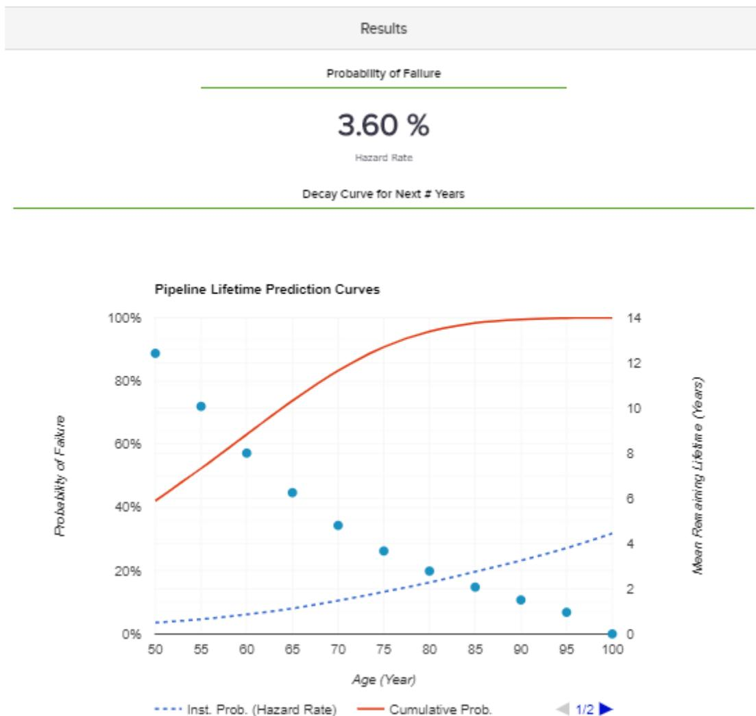
Figure 19. Results for pipe failure probability
