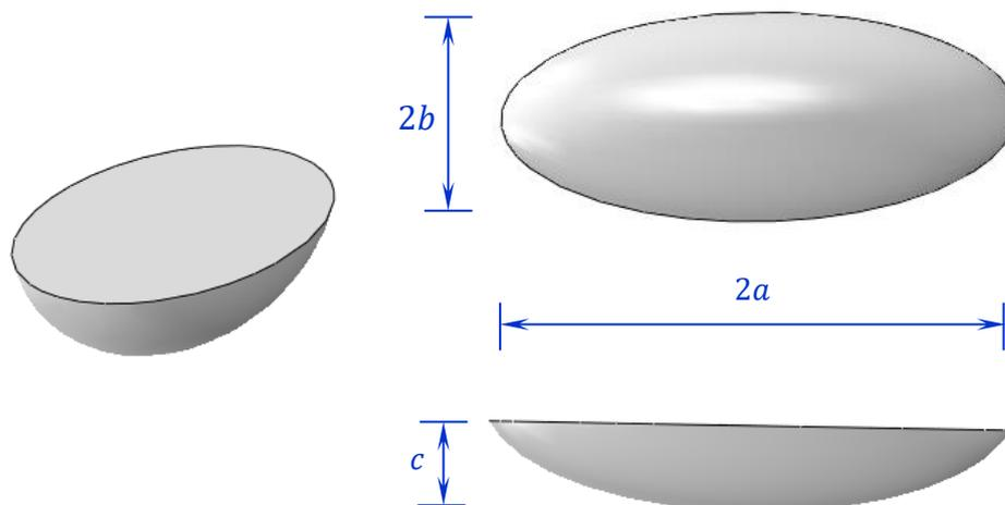
Figure 7. Geometry and dimensions of a semi-ellipsoidal corrosion patch
