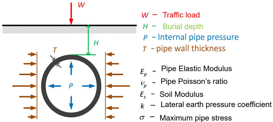
Figure 5. General variables for a buried cast iron pipe
