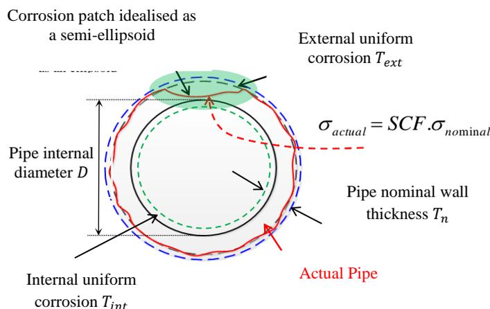
Figure 4. Cross section of a corroded pipe
