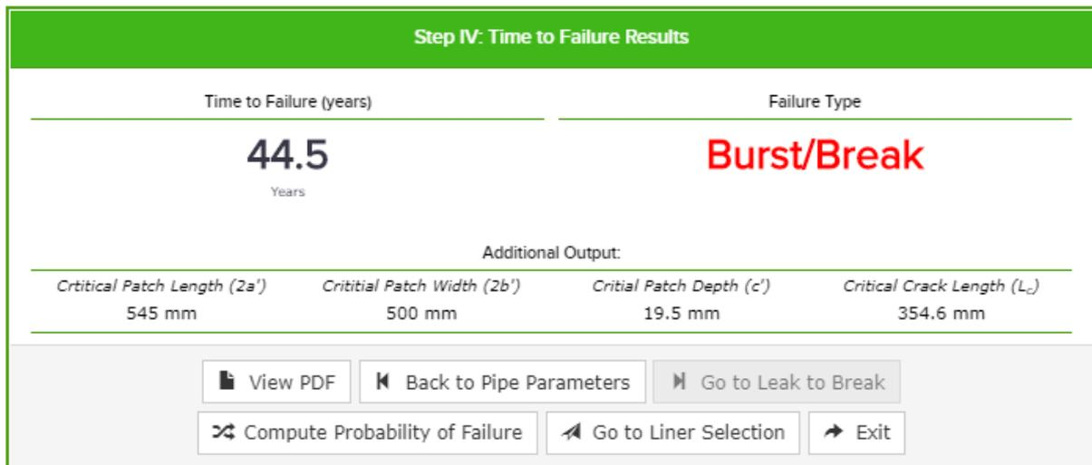
(a) Corrosion patch with dimensions ( $2a = 100$  mm,  $2b = 100$  mm,  $c = 15$  mm)
