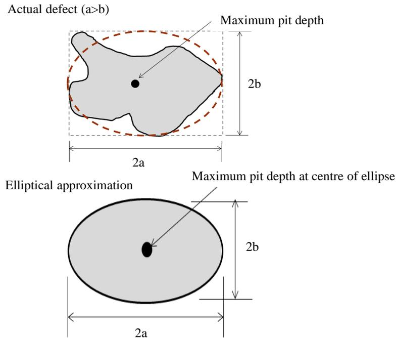
Figure 11. Approximation of irregular corrosion geometry by an ellipse
